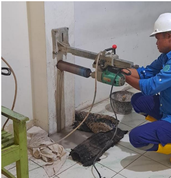
Gambar 2. Pengujian lapangan (a) hammer test (b) core drill
