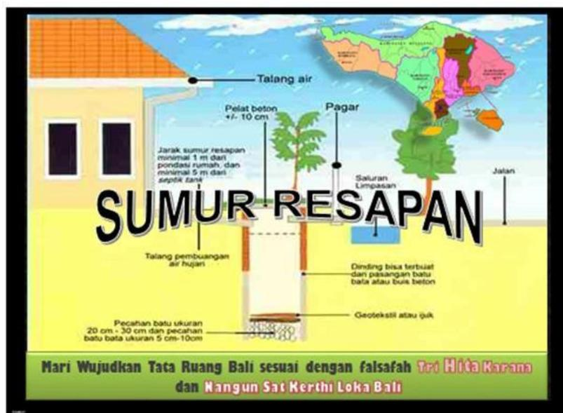
**Gambar 8 Skema Sumur resapan** (Anonim, 2020)
